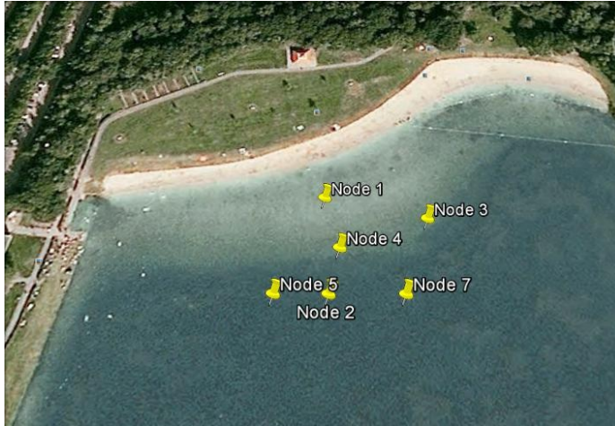
Figure 6.4: Example of network deployment on Google Earth, nodes were deployed up to a distance of 50 meters from each other
